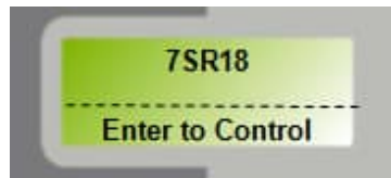
Figure 2.1-1 Relay Identifier Screen
