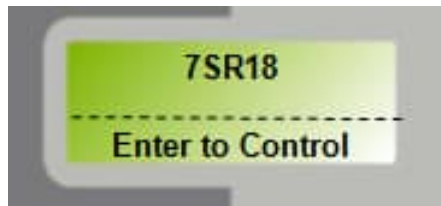
Figure 2.5-3 Typical Relay Identifier LCD Text
